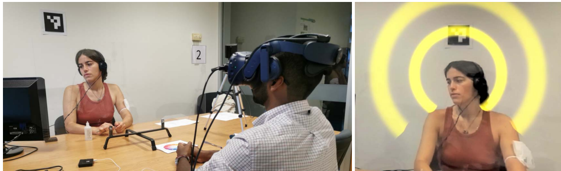
Figure 1: The AuRea system being used by a pair of participants in what we describe as the ‘Validation’ task. Left: the participant with access to AuRea via an HMD (the decoder ) observes its counterpart, wired to an ECG, watching a film clip (the encoder ). Here, the goal of the decoder is to guess the emotional state of the encoder. Right: the feedback from AuRea as seen by the decoder.
